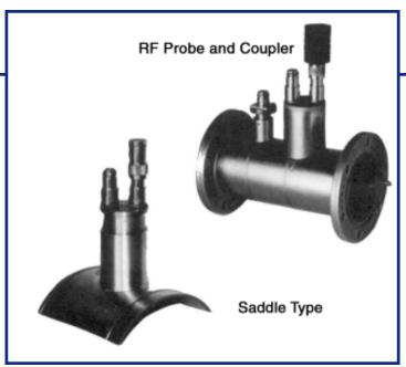
coupling. All couplers are adjustable in height and angle to select the desired value of coupling and directivity. Precision built in height and angle scales are installed for presetting. Field installable "saddle" type couplers available also.
