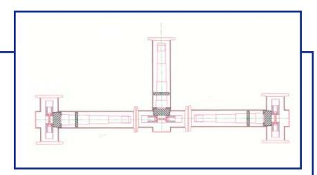
MCI's Power Combiners are used to combine as many as six power amplifiers into a single output. The combining action is accomplished by the use of precision transformer sections. The number of inputs dictates each transformer design.
