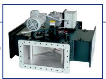
MCI series 65000 Waveguide Switches are available in motorized or manual operated configurations. The switches are manufactured from 6061-T6 structural aluminum and use silver-plated beryllium contacting gates to ensure the high isolation necessary to eliminate cross talk. All switches can handle 280kW, have low VSWR and insertion loss equivalent to the length of the waveguide.
