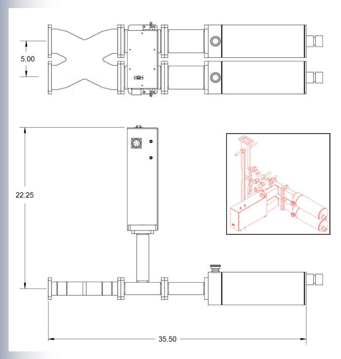
The configuration pictured is a Motorized Variable Attenuator with Hybrid input utilizing a Shunt Tee design and includes integrated Water Loads and Water Cooled Buckets for high power operation. (Inset unit water cooled with integrated output elbows)
