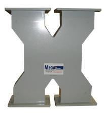
Mega Industries WR112 3dB hybrids are available as a basic subsystem building block. Quadrature, or 90 degree, equal power division hybrids are normally supplied with single flange outputs. However, dual flange outputs are available to our standards in accordance with your feed system layouts. Unequal 4.77 dB and 6 dB units are also available. If your requirements necessitate power combining or dividing in unequal ratios, contact our sales department for technical assistance.
