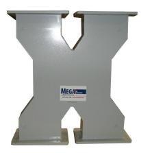
Mega Industries WR187 3dB hybrids are available as a basic subsystem building block. Quadrature, or 90 degree, equal power division hybrids are normally supplied with single flange outputs. However, dual flange outputs are available to our standards in accordance with your feed system layouts. Unequal 4.77 dB and 6 dB units are also available. If your requirements necessitate power combining or dividing in unequal ratios, contact our sales department for technical assistance.
