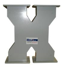
Mega Industries WR90 3dB hybrids are available as a basic subsystem building block. Quadrature, or 90 degree, equal power division hybrids are normally supplied with single flange outputs. However, dual flange outputs are available to our standards in accordance with your feed system layouts. Unequal 4.77 dB and 6 dB units are also available. If your requirements necessitate power combining or dividing in unequal ratios, contact our sales department for technical assistance.
