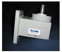
Mega Industries WR1500 Transitions to Coaxial are manufactured to precise tolerances. For laboratory testing or other low power applications, we recommend "Probe type" transitions to type "N" coaxial line; while our low VSWR "cross-bar" design provides optimum electrical performance for high power applications.
