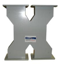
Mega Industries WR284 3dB hybrids are available as a basic subsystem building block. Quadrature, or 90 degree, equal power division hybrids are normally supplied with single flange outputs. However, dual flange outputs are available to our standards in accordance with your feed system layouts. Unequal 4.77 dB and 6 dB units are also available. If your requirements necessitate power combining or dividing in unequal ratios, contact our sales department for technical assistance.
