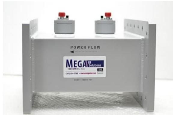
Mega Industries single, double and triple loop couplers are utilized for reflectometer measurements and power monitoring in waveguide transmission systems. With multi loop couplers, the couplers can be set at different coupling values for forward and reverse waves to optimize the dynamic range. All electrical calibration is directly traceable to the bureau of national standards.
