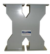
Mega Industries WR430 3dB hybrids are available as a basic subsystem building block. Quadrature, or 90 degree, equal power division hybrids are normally supplied with single flange outputs. However, dual flange outputs are available to our standards in accordance with your feed system layouts. Unequal 4.77 dB and 6 dB units are also available. If your requirements necessitate power combining or dividing in unequal ratios, contact our sales department for technical assistance.
