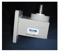
Mega Industries WR650 Transitions to Coaxial are manufactured to precise tolerances. For laboratory testing or other low power applications, we recommend "Probe type" transitions to type "N" coaxial line; while our low VSWR "cross-bar" design provides optimum electrical performance for high power applications.
