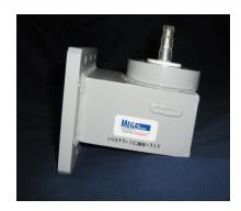
Mega Industries WR975 Transitions to Coaxial are manufactured to precise tolerances. For laboratory testing or other low power applications, we recommend "Probe type" transitions to type "N" coaxial line; while our low VSWR "cross-bar" design provides optimum electrical performance for high power applications.
