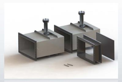
Two port Calibration Kit where two precision waveguide to Type-N female transitions are used in conjunction with a flush short circuit and a precision 1/4 Lambda waveguide section to provide a balanced response over the waveguide band.
