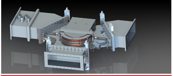
Microwave Techniques WR1800, 350kW circulator solutions place emphasis on the selection and bias point of ferrite material to minimize insertion loss and maximize isolation at the frequency, bandwidth and power level of interest. The design and power handling of a circulator is determined by the sum of the forward and reflected power, the latter being a result of any mismatch present at the output of the device. The following specifications apply to a WR1800, 350kW, UHF circulator:
