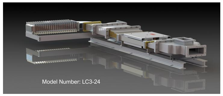
Microwave Techniques has a broad range WR650, L-Band differential phase shifting circulators. Depending on power output and mismatch conditions, cooling can be performed either by air (natural convection or forced) or liquid. Unlike junction circulators, the output mismatch has no bearing on the input match as long as the isolated ports have well matched loads. For applications of high peak power, Microwave Techniques circulators can be pressurized with air, nitrogen or SF6.
