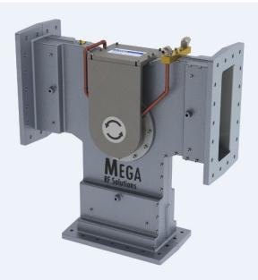
Microwave Techniques WR975 waveguide circulators are nominally optimized for RF performance at 75kW forward power. Additionally, monitor couplers are provided upon request:  $-60 \pm 2$  dB, with a Type N connector. The typical material we utilize is an Aluminum housing (A356 T1, RoHS passivated), Steel (Zinc passivated), with Copper cooling channels. We consider development in all coaxial and waveguide sizes, and custom modifications for operation at lower RF power levels.
